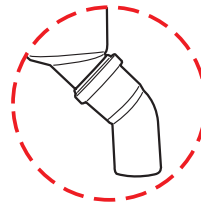
45 degree floor outlet adaptor supplied with the urinal
