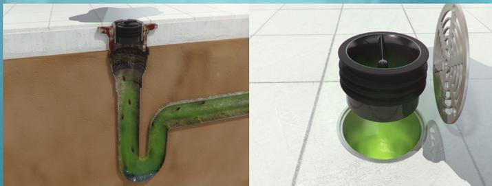
The Green Drain can help to prevent harmful radon gas infiltration through unprotected drains. The Green Drain is an economical Drain Trap Seal Device that allows water to flow down the drain while preventing Pests, Odors, and Harmful Gases/Pathogens from infiltrating the living or work space.
